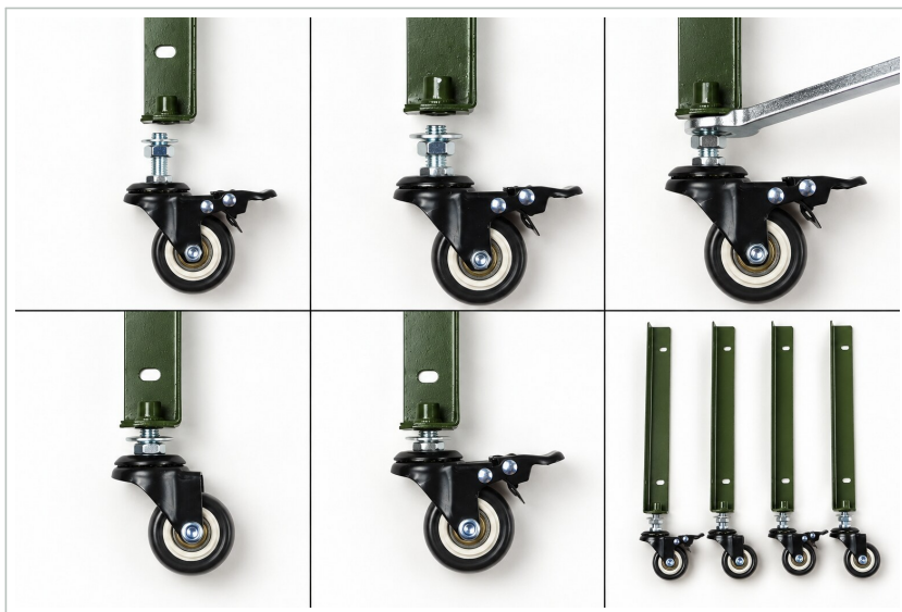
Castor stem, nut and washer order; tightening; completed legs
